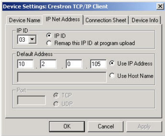
Next under the **Program View** open up the **Client** you inserted. Set the port number to **80d**. To keep implementation simple use the same signal names from the demonstration program. Your Client with signal names should look like this:
