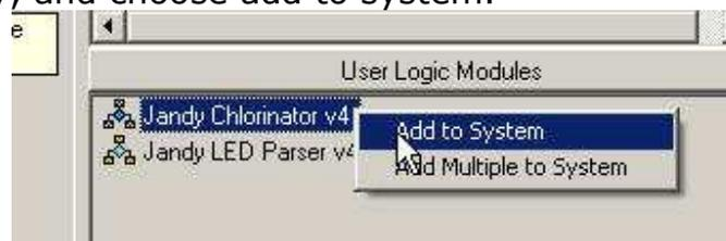
Next we need to tie the serial port the module. Since SystemBuilder will not allow you to tie logic modules to in use serial ports, we have provided specific signals on the main Jandy module to drive the LED parser module.
