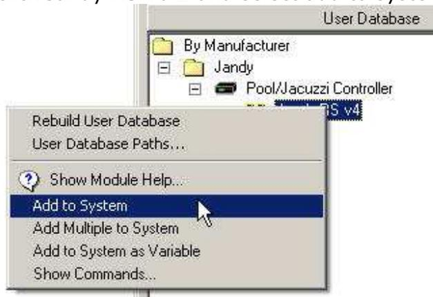
Once you have added the object to your program, you have to setup the parameters for the module. Right click on the object and select *Properties*. Then select I/O Assignment from the left hand pane. Here you should verify that the Serial Settings are correctly set to 9600,N81 with no handshaking.
