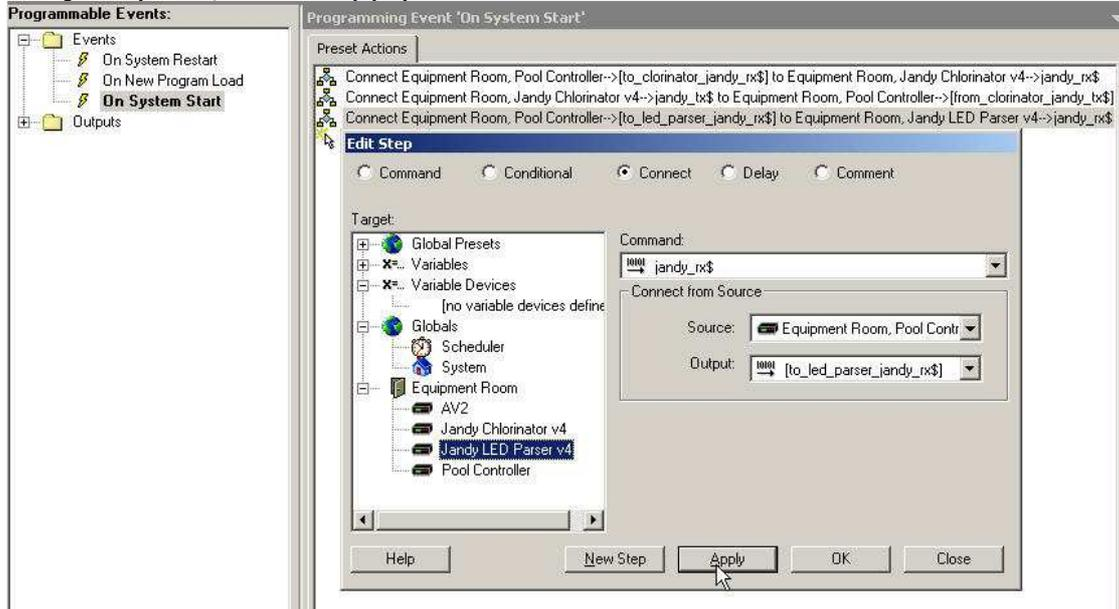
Lastly we need to connect the transmit side. Choose New step. Choose the pool controller in the target window. Next, click the connect radio button. Under the command drop down bock select from\_led\_parser\_jandy\_tx\$. Next, we will need to look underneath the command dropdown box in the connect from source area. Open source dropdown box. Choose the Jandy LED parser. Open the output dropdown box and select jandy\_tx\$. Click apply.
